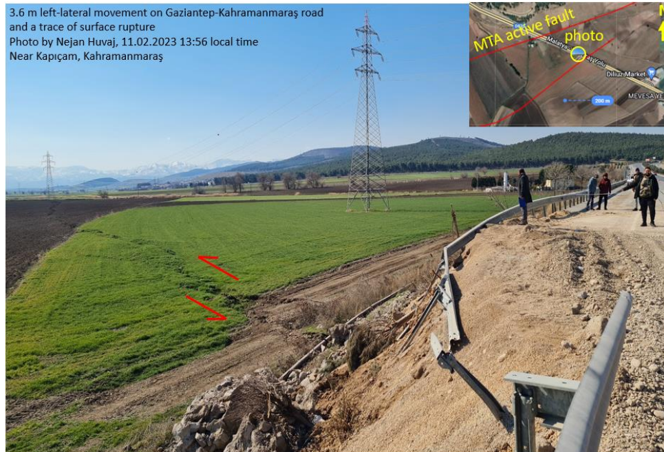
Figure 8.7. Referring to Figure 6 for the location: surface rupture observations and 3.6 m offset on Gaziantep-Kahramanmaraş road (active fault data from Emre et al. (2013)).
