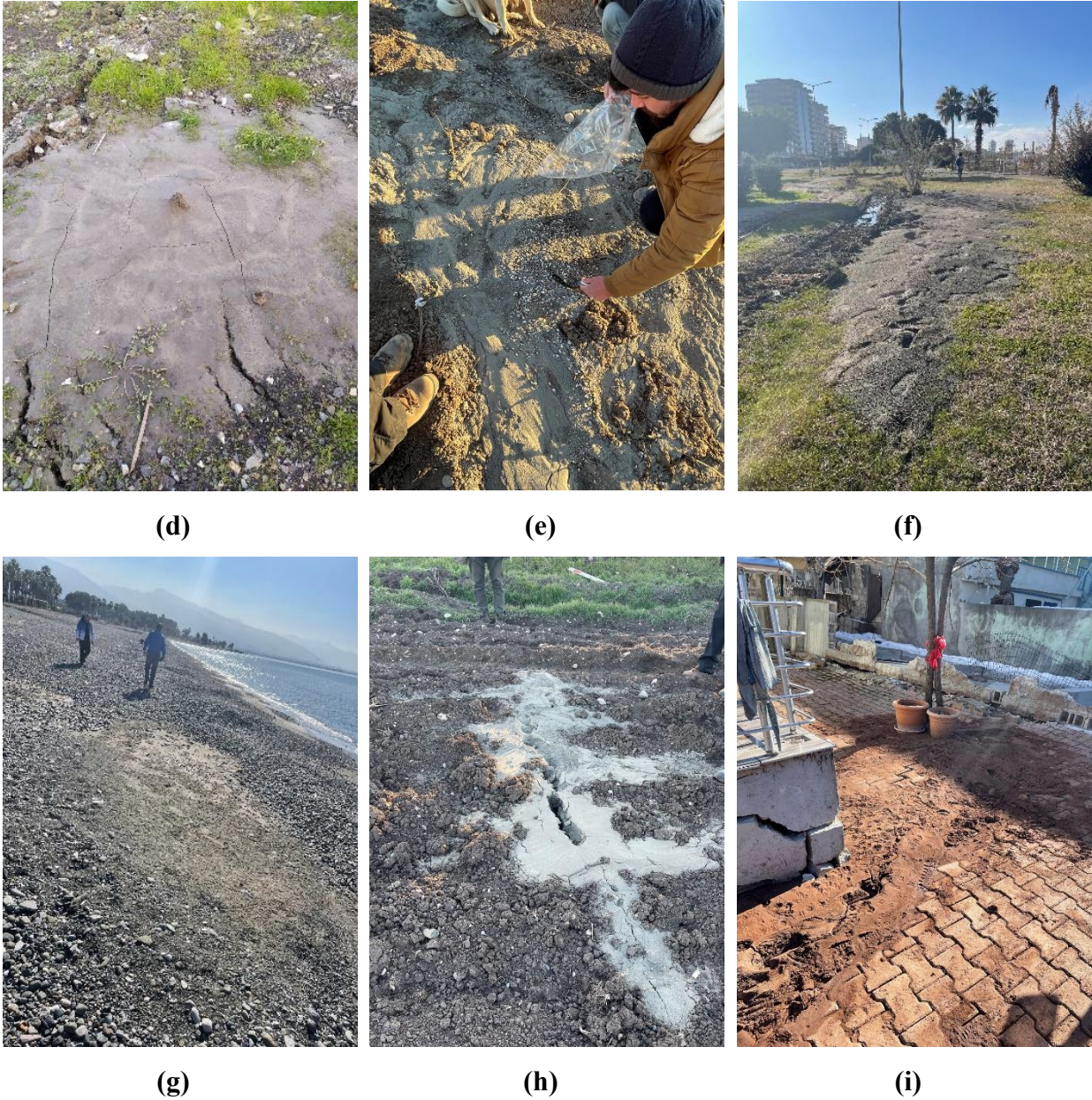
Figure 4.1. Seismic soil liquefaction-induced surface manifestation: sand boils in free field conditions: a) Hatay ( 36.36446^\circ N, 36.28147^\circ E ), b) Kumlu / Hatay ( 36.35628^\circ N, 36.39360^\circ E ), c) Fatih District / Gölbaşı / Adıyaman ( 37.78080^\circ N, 37.62888^\circ E ), d) İskenderun / Hatay ( 36.59323^\circ N, 36.18542^\circ E ), e) Emiroğlu / Kahramanmaraş ( 37.33689^\circ N, 37.04538^\circ E ), f) Çay District / İskenderun / Hatay ( 36.59133^\circ N, 36.17888^\circ E ) g) Dört Yol / Hatay ( 36.81878^\circ N, 37.17770^\circ E ) h) Emiroğlu / Kahramanmaraş ( 37.33722^\circ N, 37.04549^\circ E ) i) Gölbaşı / Adıyaman ( 37.78655^\circ N, 37.63155^\circ E )
